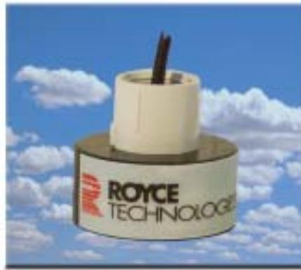
Designed specifically for the Model 2505 analyzer, this economical sensor uses a single crystal to both transmit and receive. Constructed of the same material as the 25DN; it is used in non-chemical applications where the maximum temperatures do not exceed 175° F (80° C). Its physical size allows the sensor to be inserted into a pipe with an I.D. of 3 inches. It incorporates a 3/4" 316 Stainless Steel nipple for customer supplied pipe mounting.
