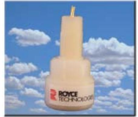
For generally harsh environment applications, this solid, Kynar sensor is made of chemically inert epoxy. It incorporates a 3/4" Kynar pipe nipple for customer supplied pipe mounting. All cables are high temperature Teflon jacketed. It can be used in chemical solutions of temperatures to 220° F (105° C).
