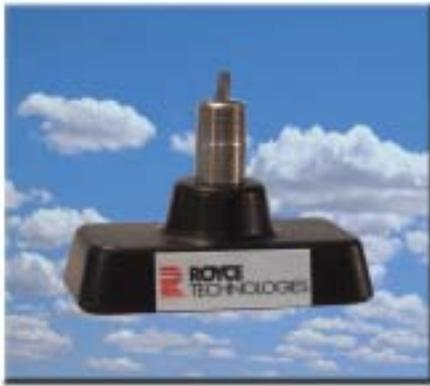
The standard ultrasonic, dual crystal sensor used with the 2501A and 2511A Interface Level Analyzers for all normal aqueous non-chemical conditions, where maximum temperatures do not exceed 175° F (80° C). It incorporates a 3/4" 316 Stainless Steel nipple for customer supplied pipe mounting.
