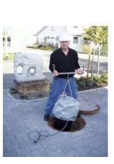
*MicroSam Ex.* The control unit can handle flow, volume event or time proportional sampling and is IP65 rated.
