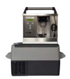
Porti 12T is useful where samples have to be refrigerated in field conditions. Able to hold a single container of either 6.4L or 10.4L or 12 x 1L bottles. The base contains a thermostat controlled compressor cooling unit that can operate on 230V, 12/24 VDC. Inside temperature +10 to -18°C. A convenient transport trolley is also available
