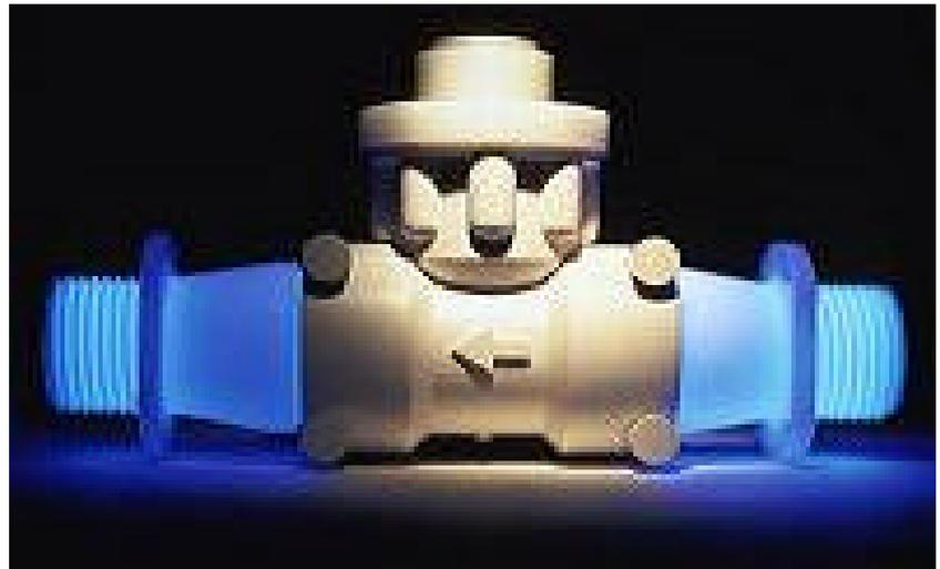
This multi-range radial flow turbine meter uses a low inertia turbine supported on robust sapphire bearings in a chemically resistant housing. Ten flow ranges (0.01 to 160 litres per minute), a choice of "plug in" fittings and individual traceable calibration make this meter one of the most flexible available. For OEM applications the fittings can be tailored to suit the installation and speed production. Custom leads or connectors are also available for quantity orders.
